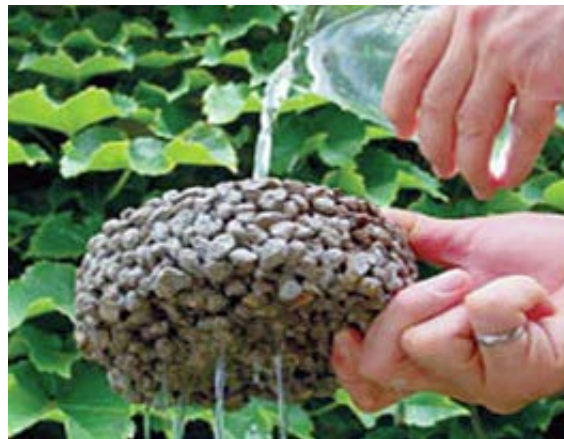
FIGURE 3-5 - Example of function of permeable pavement
